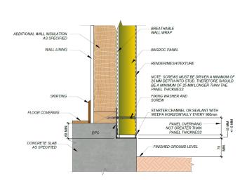
BASROC Cavity-Fix External Wall Cladding System
