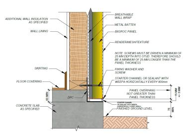
Key elements of the system as shown in figure above include:
